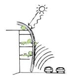
Rather than the direct entrance to the main hall through an outer door, an entrance accompanied by transition elements and preliminary places is intended. A protective facade in front of the frontal facade (south) of the building is designed in order to raise the comfort and to protect the building from radioactive effects of the direct sunlight and traffic sound.
