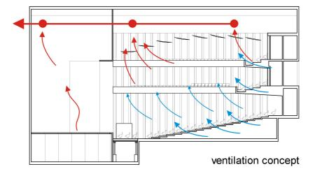
The controlled air exhaust with heat recovery makes further energy conservation possible. The supply air (cooled and dehumidified supply air) is carried out over double floor and stands in the performance hall. The air-handling system receives heating, cool and dehumidifying functions.
